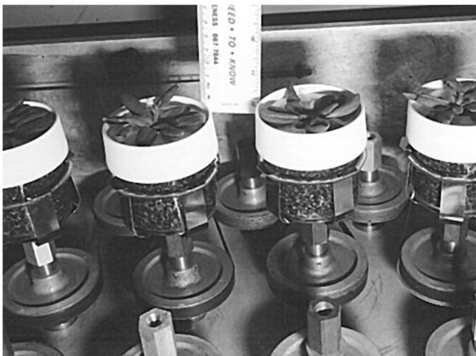
This device, called a clinostat, slowly rotates plants and can be placed sideways to investigate the effects of gravity on plant growth.
